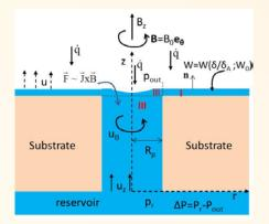
Schematic of the envisioned CPS flow arrangement in the pore level
