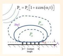
Acoustic signature of an adhered microbubble
