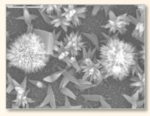
CaCO<sub>3</sub> deposits on an RO membrane.
